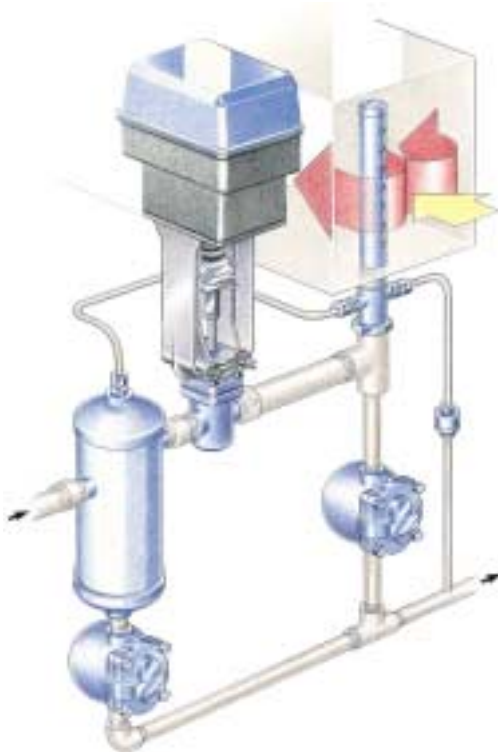
Vertical lance in horizontal duct
