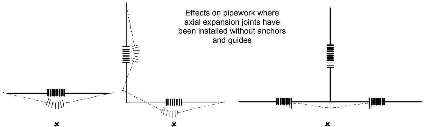
Anchors and pipe guides are essential to ensure the correct performance of the axial expansion joints. Ensure that only one axial expansion joint is installed between anchors.
